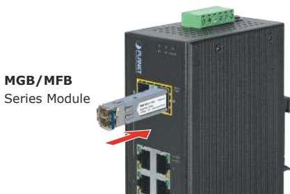
Figure 3-1: Plug-in the SFP Transceiver
