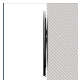
Ultra-slim design mounts screen only 30mm (1.2") from wall
